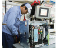
Large-sized circuit breakers produced at the Kami factory. The finished products weigh several tens of kilograms
