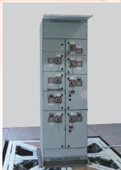
Vibration test based on IEC requirement IEC に基づいた振動試験
