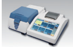
Loopamp Turbidity Measurement Device — a genetic testing device for viral infection screening
