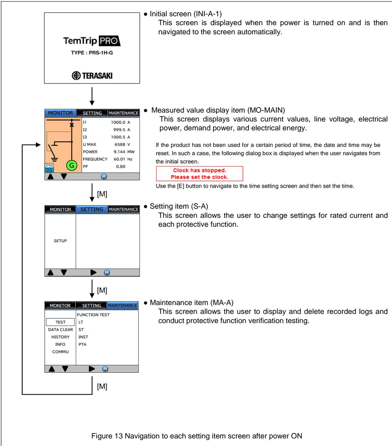
Figure 13 Navigation to each setting item screen after power ON
