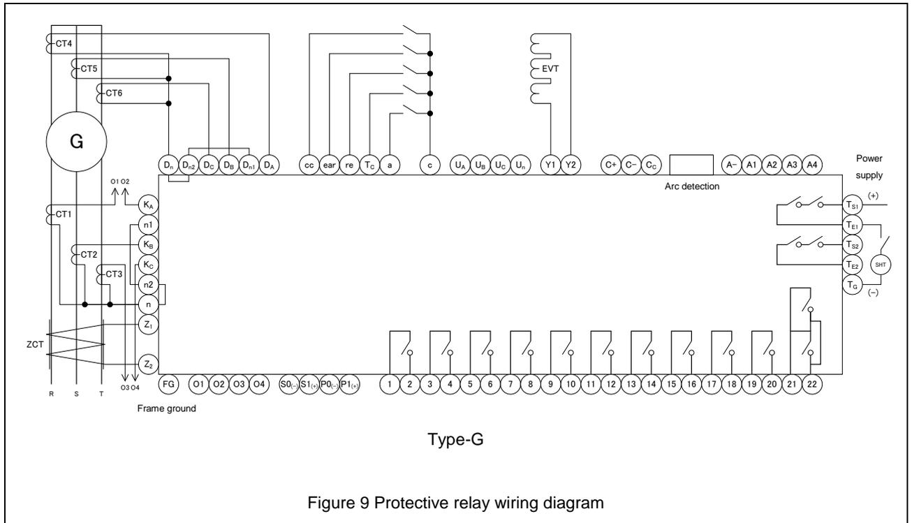
Note: The wiring diagram illustrates the wiring of the protective relay with all the options mounted.
