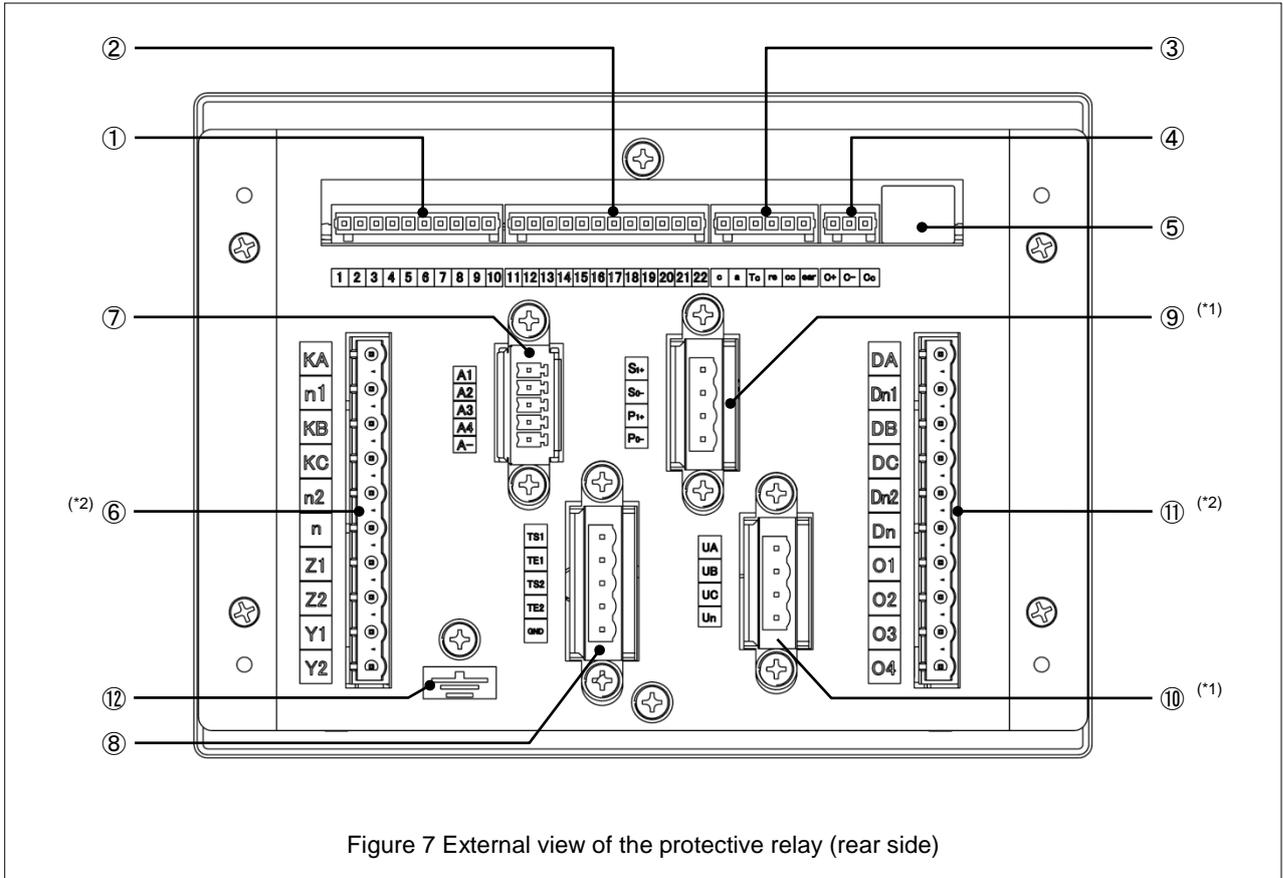
Figure 7 External view of the protective relay (rear side)
