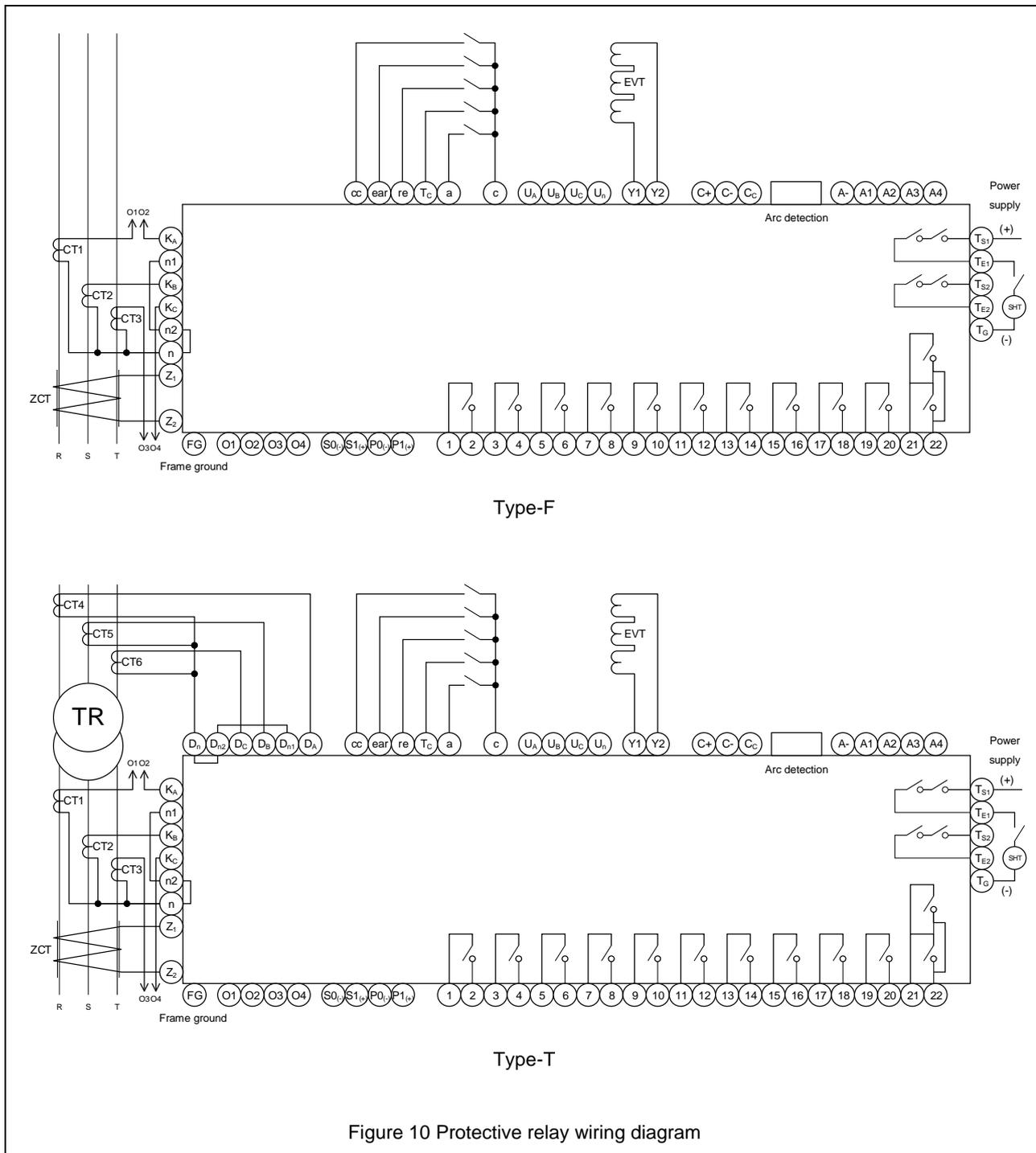
Figure 10 Protective relay wiring diagram
