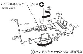
る位置までハンドルを回します。 Rotate the handle until the screw head is visible at the handle catch
