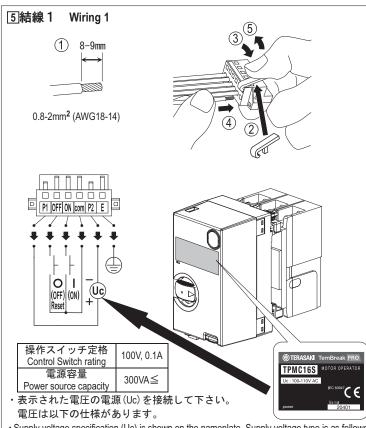
· Supply voltage specification (Uc) is shown on the nameplate. Supply voltage type is as follows. 電圧の種類 Supply voltage type 100/110V AC 200/220V AC 230/240V AC 24V DC
